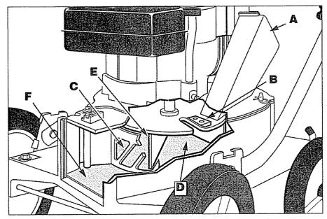
Figure 21: Cutaway view. (Blower deflector removed for clarity.)
